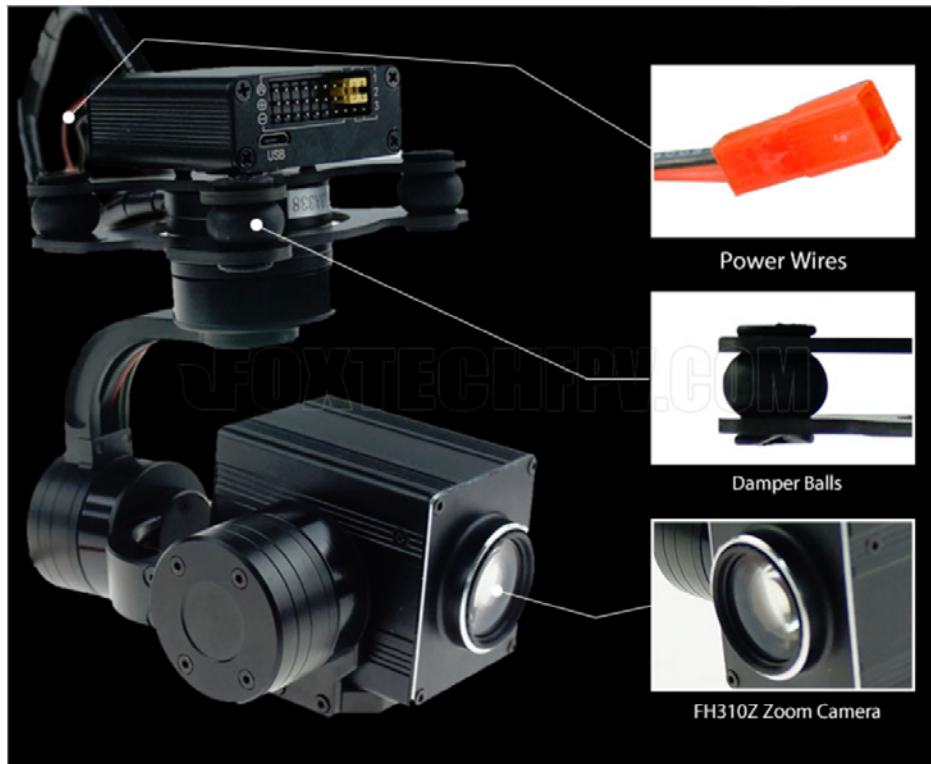
Figure 36. FH310Z Camera with Gimbal System (Foxtech, 2017)
